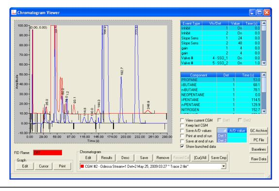
Figure 2-7. The Chromatogram Viewer displaying an archived chromatogram
